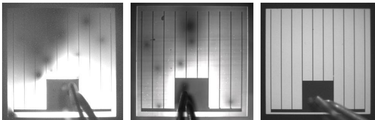
Figure 3.5. Representative electroluminescence images of the regular (left) and QD (middle) thin-film cells in comparison to that of a substrate based cell (right). The thin-film cells showing point defects and misfit dislocation lines typically require currents in the 40-80 mA while the substrate based cells showing homogeneous luminescence require currents in the 0.5-5 mA range to obtain an image.
