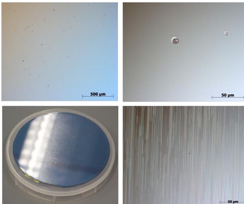
Figure 2.1. Typical particle-like and oval defects observed on all epi-structures of the first batch (upper images) and high density of misfit dislocations on the epi-structures with 50 and 100 layers of QDs (lower images).
